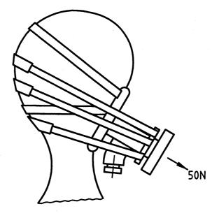
Figure 1 — Typical arrangement for testing connections
